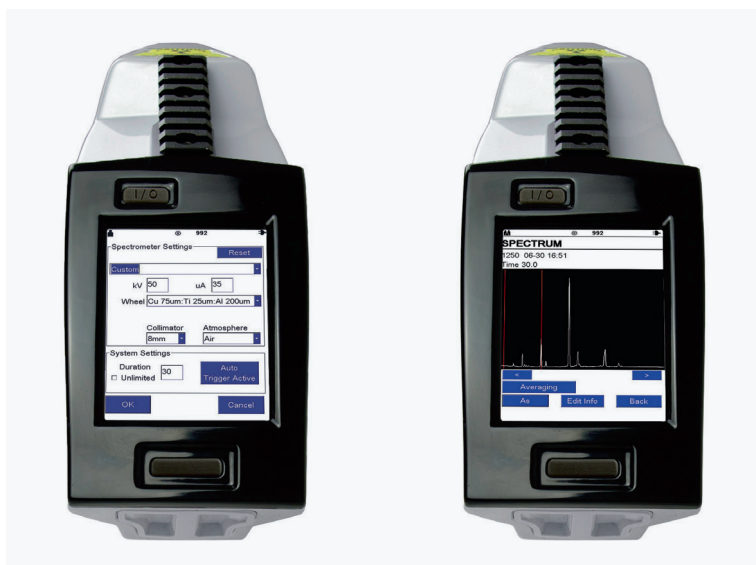
Figure 1 TRACER 5 interactive user interface for control and results
