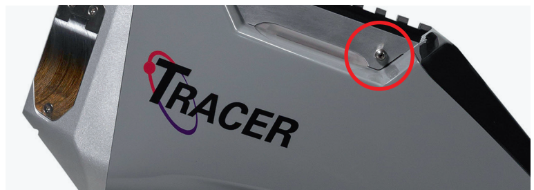
Figure 6 Port connection (red circle) to purge with helium
