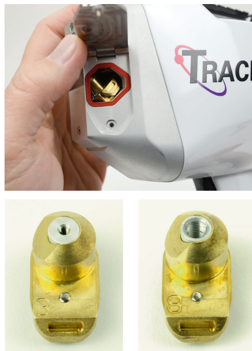
Figure 4 Portal for user changeable collimators (3 mm bottom left and 8 mm bottom right) and custom filters
