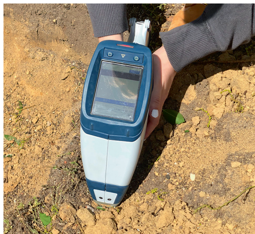
Soil analysis with the S1 TITAN
