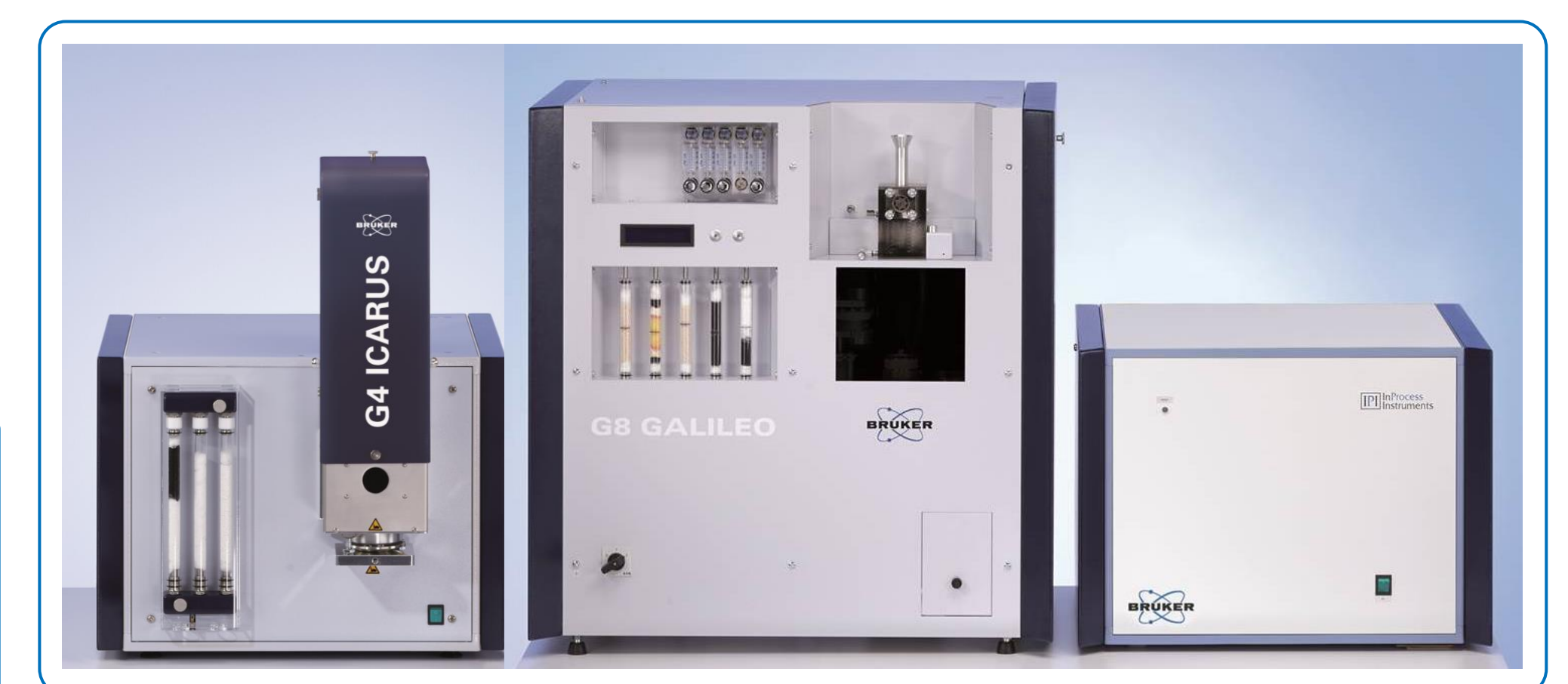
Figure 2. Bruker G4 Icarus HF CS analyzer (left) and Bruker G8 Galileo ONH analyzer (middle) coupled to a MS detector (right).
